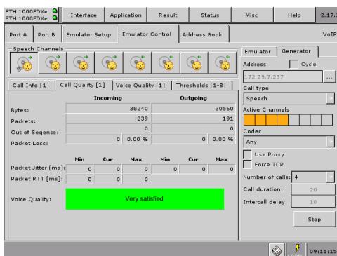
Fig. 20 A total of 8 VoIP calls can be generated through the CMA 3000 Ethernet's two test ports. The voice quality evaluation is presented for one call if the Voice Quality Measurement option is installed.
