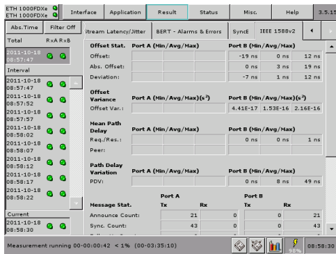
Fig. 15 Comprehensive IEEE 1588 v2 statistics on offset and offset variance, path delay variation, messages and clock state transitions.
